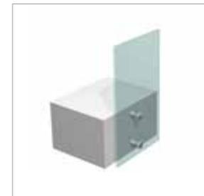
Easy Glass® MOD 0749, the first adjustable standoff for glass railings, is Q-railing's solution for what has historically been a vexing problem. Walls and other surfaces are rarely perfectly straight. The MOD 0749 easily straightens glass panels on site, with absolutely no on-site welding required. Featuring a 2-way-fix connection, the base also has space for a mechanical anchor system.
